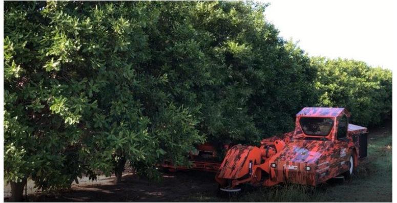
Figure 7: Tree shakers are used to dislodge mature nuts that have not fallen naturally.
